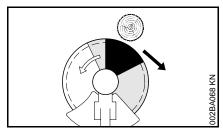
The risk of kickout is highest in the black area of the blade: Do not use this area of the circular saw blade for cutting.
