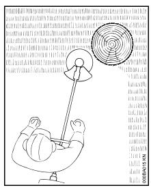
For trimming around fence posts, trees, etc. - less risk of damaging tree bark.
