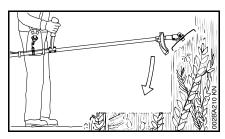
To cut wild growth and scrub, lower the shredder blade down onto the growth to achieve shredding effect – do not use the cutting attachment above waist height.
